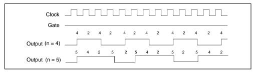
Figure 2-35. Mode 3 Timing Diagram
